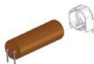
1) Assemble capacitor and holder
