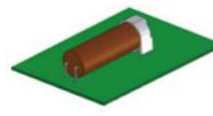
3) Mount capacitor and holder (reflow soldering)
