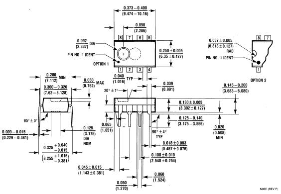
Molded Dual-In-Line Package (N) Order Number LM392N NS Package Number N08E
