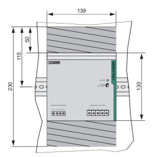
Mounting position: Installation depth 190 mm (+ DIN rail)
