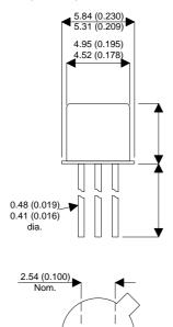
ტ 3 Bipolar PNP Device in a Hermetically sealed TO18 Metal Package.
