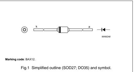
The BAX12 is a controlled avalanche diode fabricated in planar technology, and
