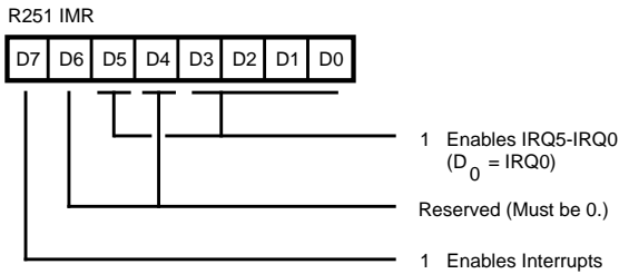
Figure 26. Interrupt Mask Register (FB H : Read/Write)
