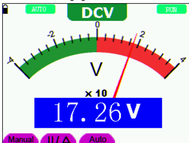
Figure 21: DC Voltage Measurement
