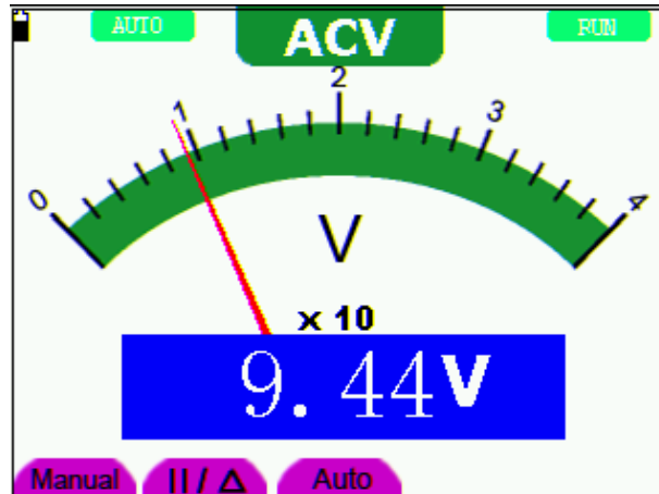
Figure 22: AC Voltage Measurement
