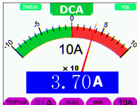
Figure 28: DC Current Measurement for <10A
