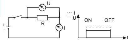
Voltage-current characteristic when switching a relay coil (fig. 2).
