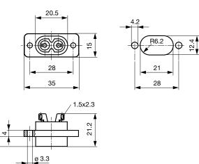
Solder terminals for wires
