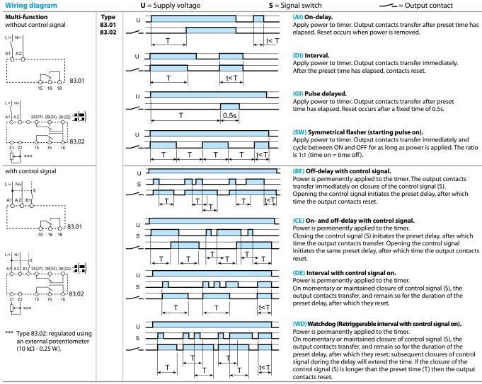
NOTE: The timing function must be set when the timer is de-energised. Or for the 83.02/52, when the contact mode selector is in the OFF position.
