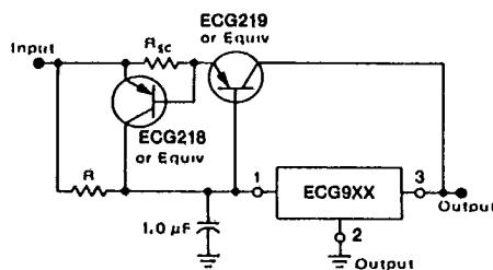
The circuit can be modified to provide supply protection against short circuits by adding a short circuit sense resistor,  $R_{SC}$ , and an additional PNP transistor. The current sensing PNP must be able to handle the short-circuit current of the three terminal regulator. Therefore, a four-ampere plastic power transistor is specified.
