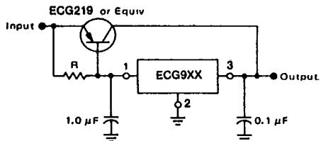
The ECG9XX series can be current boosted with a PNP transistor. The ECG219 provides current to 5.0 amperes. Resistor  $R$  in conjunction with the  $V_{BE}$  of the PNP determines when the pass transistor begins conducting. This circuit is not short-circuit proof. Input-output differential voltage minimum is increased by  $V_{BE}$  of the pass transistor.
