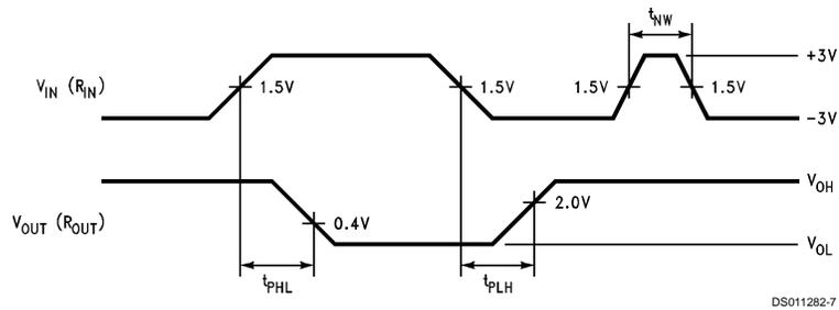
FIGURE 4. Receiver Propagation Delays and Noise Rejection
