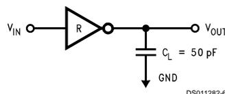
FIGURE 3. Receiver Load Circuit
