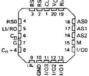
Four I/O ports (I/O 0 thru I/O 3) are provided for parallel loading of word A and/or word B into their respective registers. These same ports also serve as bus driving outputs for the ALU/accumulator results (Fj). Two additional I/O ports (RI/LO and LI/RO) are provided to allow expansion of the accumulator for words greater than four bits in length.
