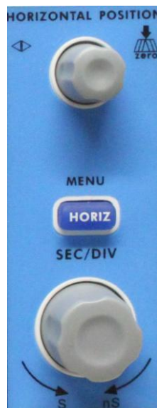
Fig. 11 Horizontal Control Zone
