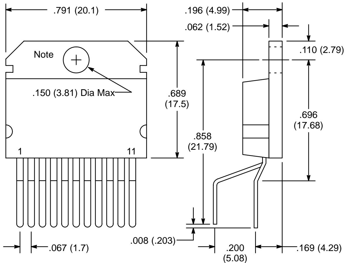
**NOTE:** Tab connected to Pin6
