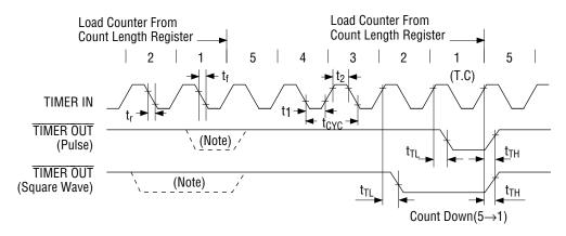
**Note:** Periodically outut according to the output mode (m1=1) programming contents.
