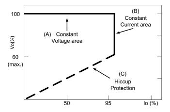
Typical LED power supply I-V curve
