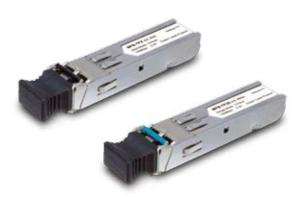
The MFB family consists of Small Form Factor Pluggable (SFP) transceiver modules that are specifically designed for high performance integrated duplex data link over single mode optical fiber. These transceiver modules are compliant with the SFP Multisource Agreement (MSA) and hot pluggable. These modules offer an easy way to be installed in SFP MSA compliant ports at any time without the interruption of the host equipments operation.
