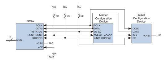
Figure 5–3. Altera FPGA Configured Using Two EPC2 or EPC1 Configuration Devices Note (1)
