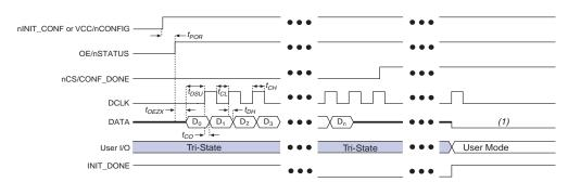
Figure 5-5. Timing Waveform Using a Configuration Device
