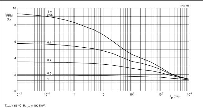
$I_{amb}$  = 55 °C;  $R_{th j - a}$  = 100 K/W.  $V_{RRMmax}$  during 1 –  $\delta$ ; curves include derating for  $T_{j max}$  at  $V_{RRM}$  = 1000 V.
