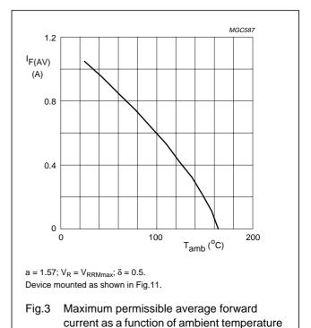
(including losses due to reverse leakage).
