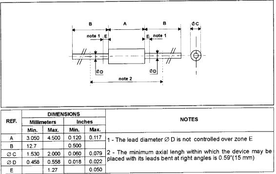
Cooling method : by convection and conduction Marking: clear, ring at cathode end. Weight: 0.15g
