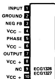
**ECG1328** 10-Pin SIP-M See Fig. L66
